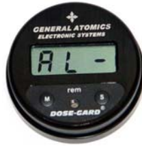
Fig 2.5 Alarm Acknowledge Mode Display
